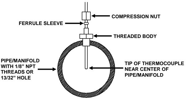
Figure 2. Thermocouple Mounting
